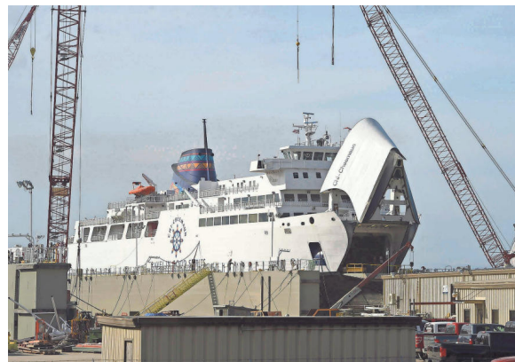
PHOTOS BY STEVE REINKE/SUBMITTED The MS (Motor Ship) Chi-Cheemaun is in port for a required five-year inspection at Fincantieri Bay Shipbuilding Co., Sturgeon Bay. It is a RO-LO (roll on/roll off) ferry — vehicles roll onto the ferry and roll off. A unique feature is that the bow is lifted to unload vehicles, as seen here. The ferry currently resides in Bay Ship's floating dry dock. To see more photos of the Chi-Cheemaun, go to the gallery at www.greenbaypressgazette.com .
